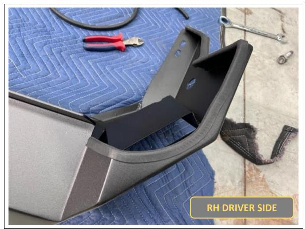
15. Fit pinch weld over the edges of each bar wing as shown. This protects the vehicle tub during installation of the bar. Cut to length with side cutters.
