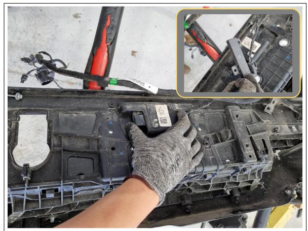
10. If equipped, remove the keyless entry RF module from the middle of the bumper and set aside.
