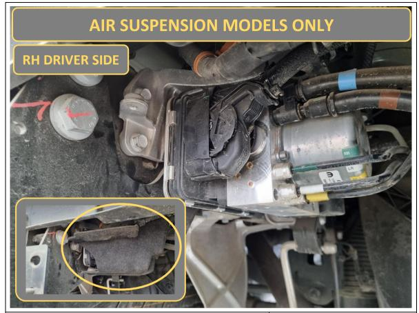
2. If vehicle is equipped with air suspension, remove the splash shield covering the air suspension module on the RH driver side chassis rail, next to where the tow bar attaches to the chassis.
