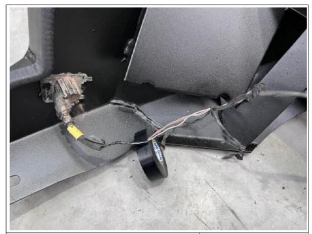
20. Cover exposed wires with electrical tape.
