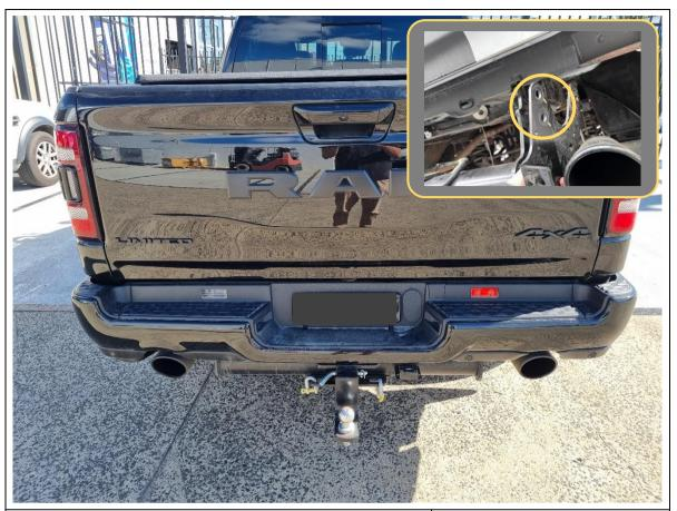
4. Remove RAM factory bumper, and if fitted, the pull out step. Re-fit the factory tow bar leaving the large M16 bolts on the sides out for later.
