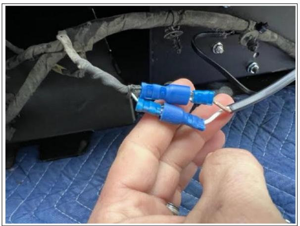
21. Wire in the new number plate lights to existing wires. Use crimp connectors (shown above) or solder/heat shrink wires together.
