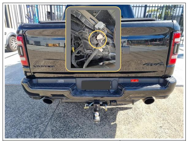
1. Unplug and unclip all of the bumper and tow bar harnesses inside the rear bumper.
