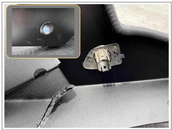
16. Use an industrial grade adhesive silicone or double sided tape to secure the sensor housings to the inside of the rear bar.
