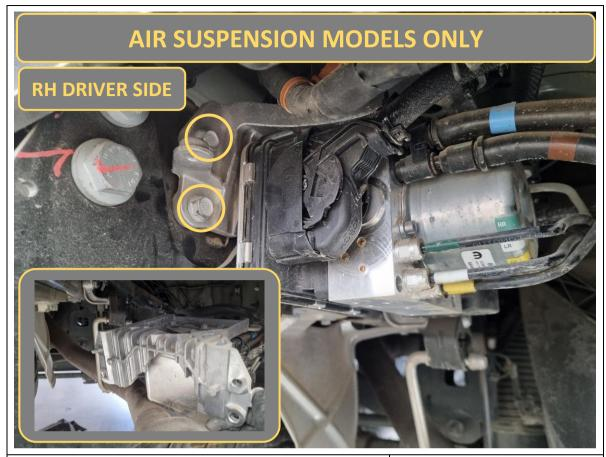
3. If vehicle is equipped with air suspension, remove the 4x M8 bolts holding the air suspension module to the chassis. Let the module hang (and rest on the exhaust if it's not hot) for now.
